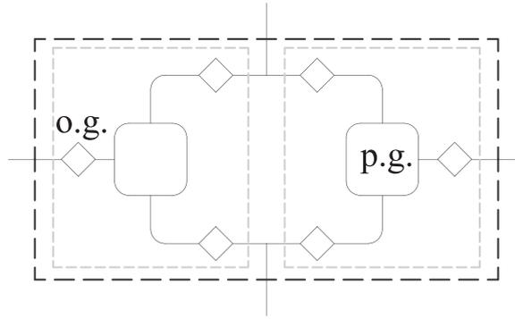
**Fig. 2.** The general PSU consists of two three-port differentials, each one made up of a planetary gearing (p.g.) and three ordinary gears (o.g.). There are two pairs of homologous joints, i.e. ordinary gears linked to the same main shaft.
