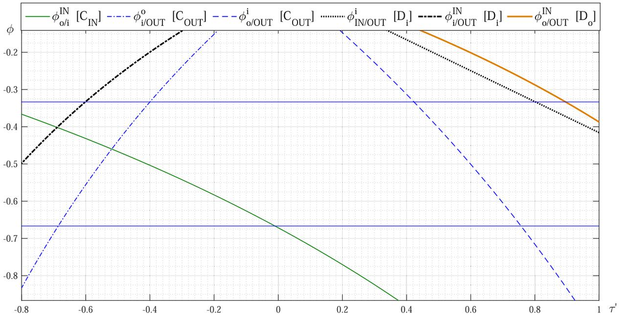
Fig. 5. Design-chart for  $A = -0.8$ ,  $A_v = 3.6$ ,  $A_i = 0.47$  and Willis' ratios within the range  $[-1/3, -2/3]$ . It represents the characteristic functions  $\phi$ . Their superscripts and subscripts define the carrier, ring and sun position.
