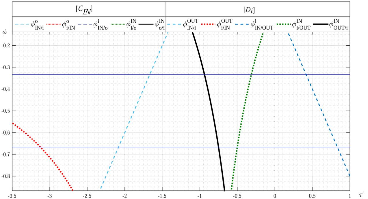
Fig. 10. Design chart for the PS-CVT with  $A = A_o = -3.5, A_i = -1$  and Willis' ratios within the range  $[-1/3, -2/3]$ . It represents the characteristic functions  $\phi$ . Their superscripts and subscripts define the carrier, ring and sun position.
