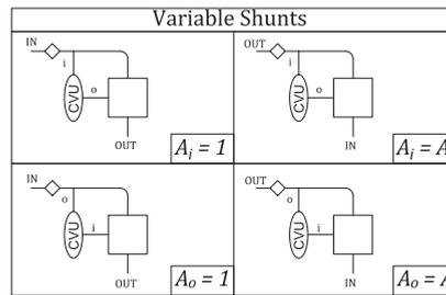
**Fig. 9.** Variable shunt transmissions: Output-splits (on the left) and input-split (on the right).
