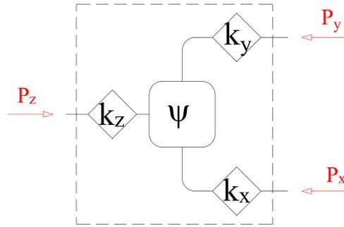
**Fig. 3.** Basic layout of a three-port differential, which is made up of one planetary gear train and three fixed ratio joints. Any power is assumed positive if entering.
