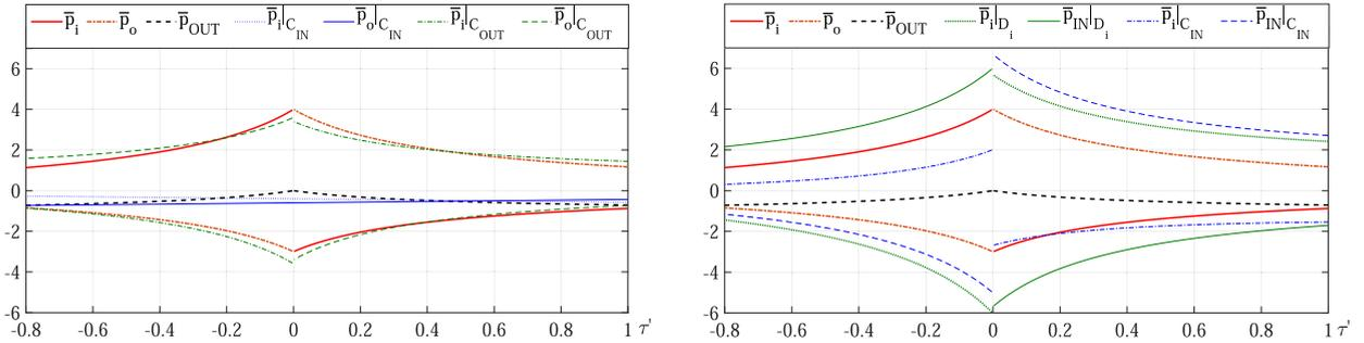
Fig. 7. Internal power flows of the  $C_{IN}-C_{OUT}$  (left) and  $D_i-C_{IN}$  (right) layouts for the transmission of the example of Section 4 ( $A = -0.8, A_v = 3.6, A_i = 0.47, \eta_v = 0.75$ ).
