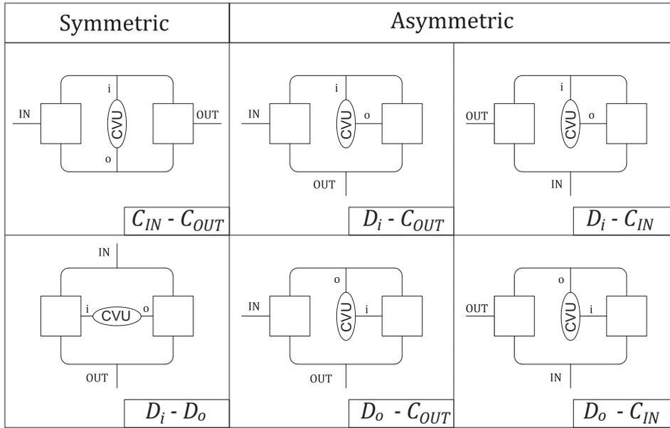
Fig. 4. Functional schemes for compound power-split transmissions. The fundamental layouts are: Cross Bridge, Direct Bridge and Asymmetric Bridge.
