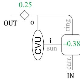
Fig. 11. Final constructive scheme of the transmission designed in Section 4.1.
