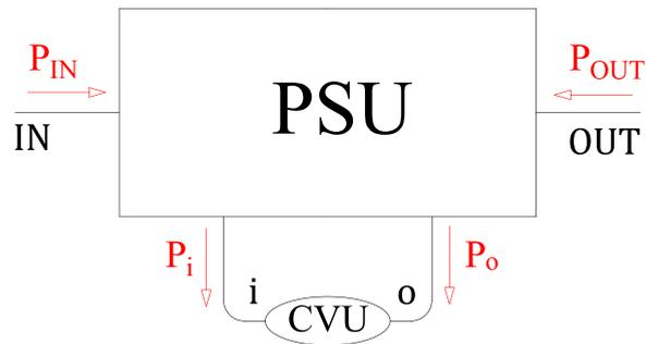
Fig. 1. Basic layout of a power-split CVT, which is made up of a PSU and a CVU. The represented power flows are assumed positive.
