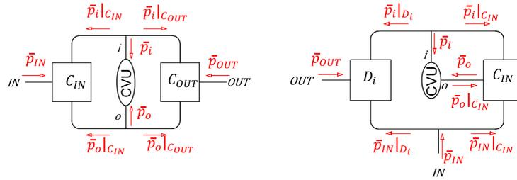
Fig. 6. Selected functional schemes for the transmission of the example of Section 3.3. According to Fig. 1 and Fig. 3 all the represented power flows are assumed to be positive.
