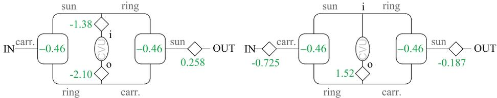
**Fig. 8.** Eligible final constructive schemes of the transmission designed in Section 3.3. For  $\tau_{i_m} = +2.5$  all the fixed ratios would be positive.
