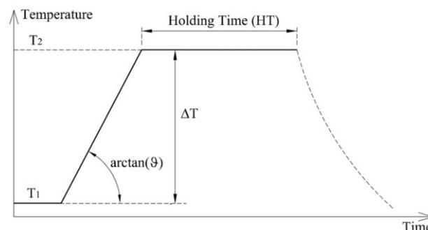
FIG. 2. SCHEMATIC REPRESENTATION OF A TEMPERATURE-TIME PROFILE OF DYNAMIC IRREVERSIBLE THERMOPORATION THERMAL PROCESS
